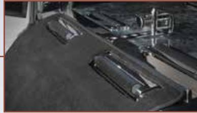
The MKT Stratford features 90-degree rear rollers, rear carpet bumper protector, and a quick-release adjustable bier pin.
