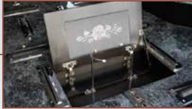
Floor hardware includes a standard Urn Holder, front dual bier pin plates, ten rollers and eight skid bars.
